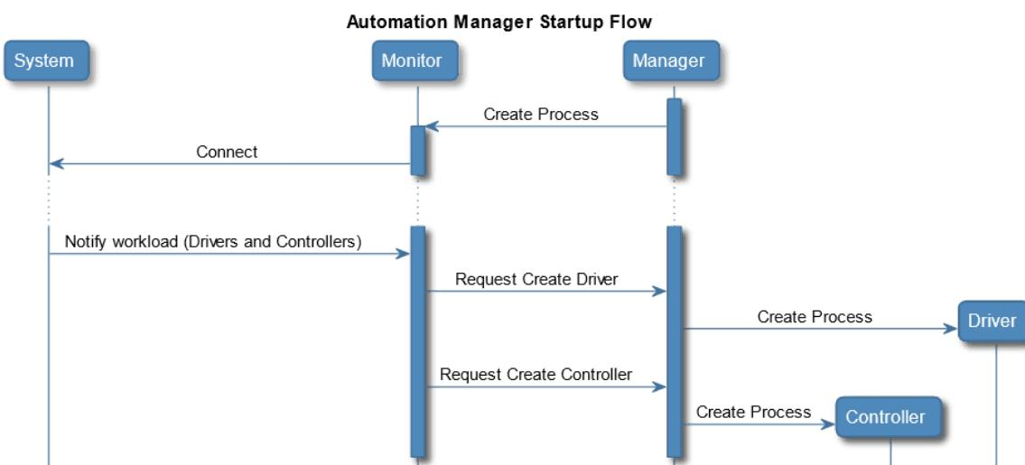
The Manager process is the parent process, responsible for orchestrating the application. The Manager will spin up a Monitor subprocess, which interacts with the MES system and retrieves all the needed configurations and dependencies. The Monitor will forward to the Manager what are the processes for the Driver and Controller that need to be spun up. The Driver and Controller then start and have their own runtime cycles.
