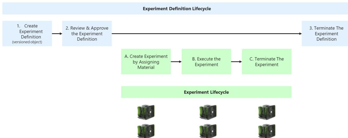
The Experiment object that represents the running Experiment Definition instance and that always requires a Material follows the lifecycle as shown in the image below and described in the table immediately after:
