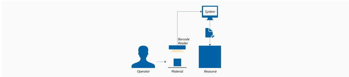
This example illustrates the machine domain and the domain of process configuration (which knows the barcode and the recipe to use). The role of equipment integration is to interact and interface with these two systems to generate value.
