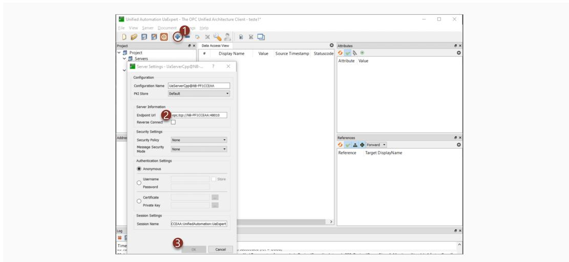
4. Select Connect, and on the address space, go for `BuildingAutomation > FurnaceXml`, and drag and drop Temperature and TemperatureSetPoint to the Data Access View
