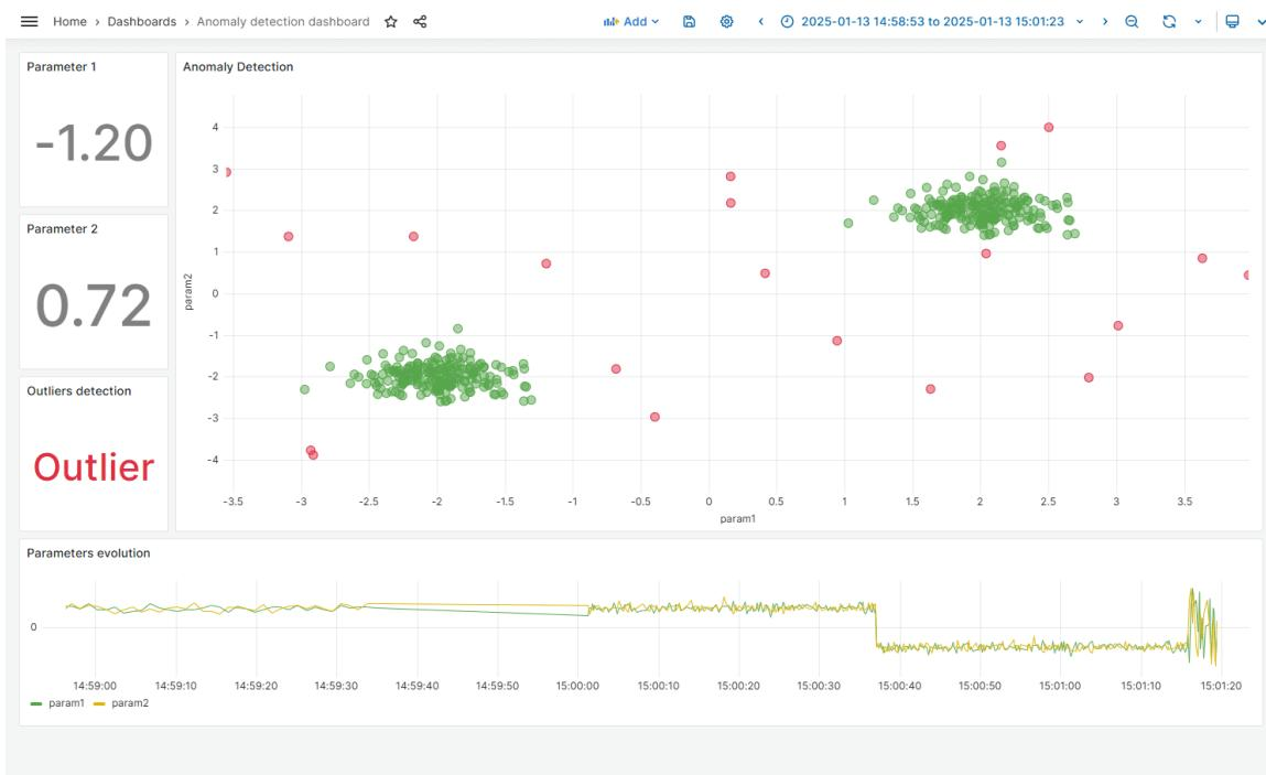
Here, we can immediately observe the abnormal data points by looking into the scatter plot and how the ML Model efficiently detects the outliers. We can see from the time-series the period when the abnormal behavior started.
