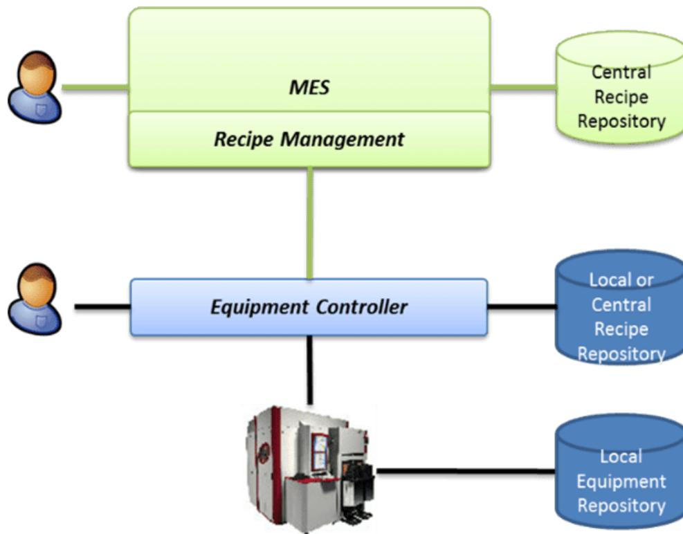
**Recipes** can be stored and edited centrally in the **MES**, but often it's the case that they can be edited only in the equipment or equipment controller. The system must therefore support the download and upload of **Recipes** from/to equipment.
